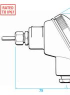
block. Suitable for 2, 3 or 4 wire simplex assemblies or 2 or 3 wire duplex assemblies only. Supplied with a 20mm x 1.5mm ISO plastic pinch gland on the cable entry for cables from 6mm to 14mm diameter. Terminal head temperature rated to 150°C. \* A smaller version of this connection head is also available and is
