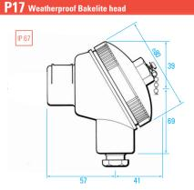
Weatherproof Bakelite plastic screw top terminal head with tube entry and cable entry at a right angle to each other. Suitable for use with TBB terminal blocks. Supplied with a 1/2 in BSP tube entry and a 20mm x 1.5mm ISO cable entry. A plastic cable gland is supplied suitable for cables from 6mm to 14mm diameter. Terminal head temperature rated to 150PC. \*A smaller version similar to the PI7 is also available and is referred to as P16.
