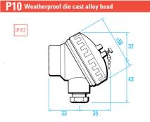
Weatherproof die cast alloy, epoxy coated, screw top terminal head with the tube entry and cable entry at a right angle to each other. Suitable for simplex and duplex assemblies. Suitable for use with TBCM terminal blocks. Supplied with a 16mm x 1.5mm ISO tube entry and a 16mm x 1.5mm ISO cable entry. A metal cable gland is supplied suitable for cables from 3mm to 8mm diameter. Also available in a range of colours including Green, Brown, Black, Pink, Orange Purple and White.
