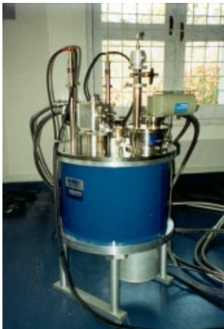
Figure 3. Photograph of a fully assembled magnet
