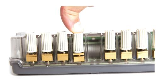
Connect your probes by simply pushing on the terminal top and insert wires of up to 3 mm or 10 AWG diameter and compensated thermocouple connectors.
